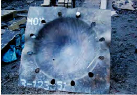
**ARMOX 440T** has the highest toughness in our range. Its superior toughness makes this steel a common choice for applications with high requirements on blast protection. The purity and composition of the steel also makes the steel easy to process, including excellent properties for welding and bending.
