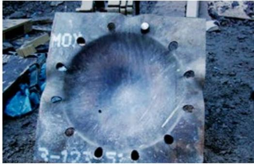
**ARMOX® 440T** has the highest toughness in our range. Its superior toughness makes this steel a common choice for applications with high requirements on blast protection. The cleanliness and chemical composition of the steel also makes it easy to process, including excellent properties for welding and bending.
