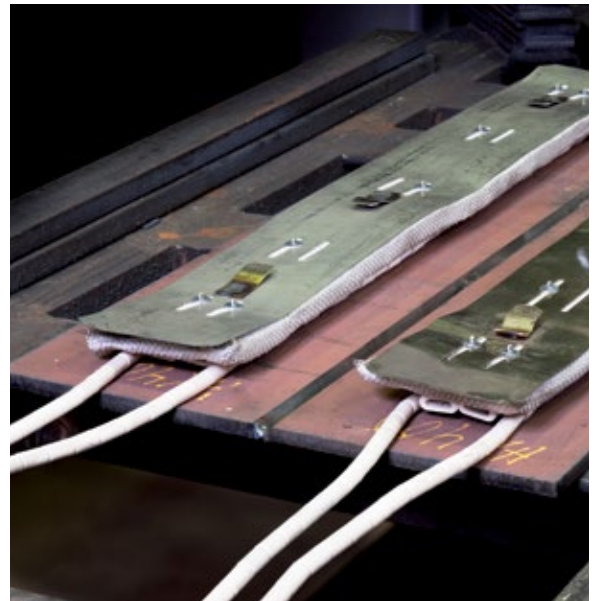
Figure 4 Using preheating blankets.
