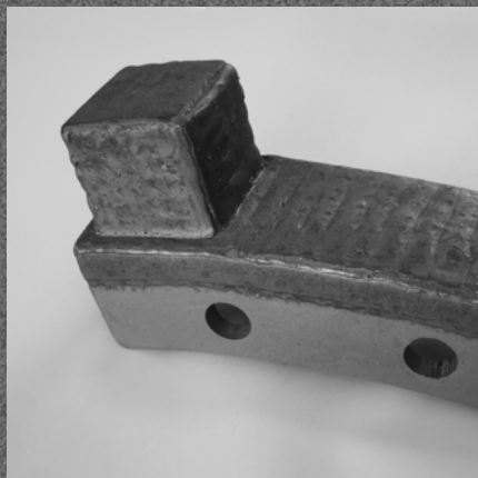
Rotor caps for aluminum recycling
