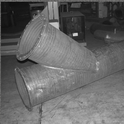
Y-shaped pipes for cullet glass
