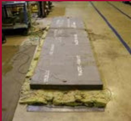
5. Put on the plate and place thermal couples which will log the temperature over time
