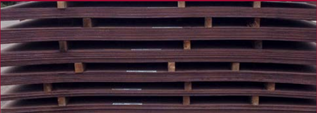
Figure 13b: Improperly stacked plates
