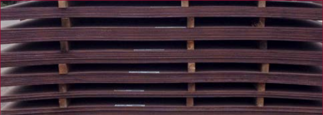
Figure 13a: Properly stacked plates.
