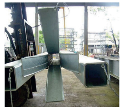
Fig. 11. Example of extreme corner cracking in a rectangular hollow section during hot-dip galvanizing [5]
