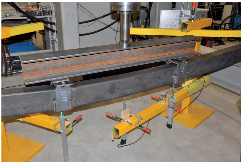
Figure 1. Bending test and corresponding failure mode for tubular S700MH member.
