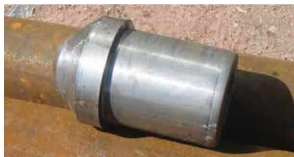
Figure 12. Example of an adapter between the striker of the hydraulic ram and the pile during impact.
