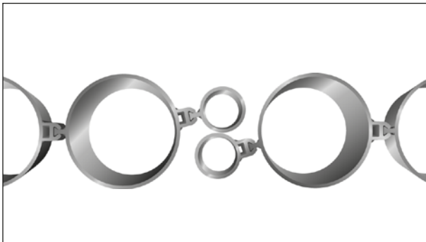
Figure 23. Joining wall ends by overlapping
