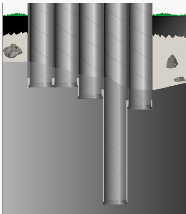
Figure 30. Ending of a connector when a pile is required to be installed at a lower level than the previous one.
