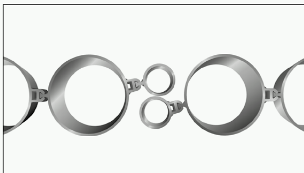
Figure 23. Joining wall ends by overlapping
