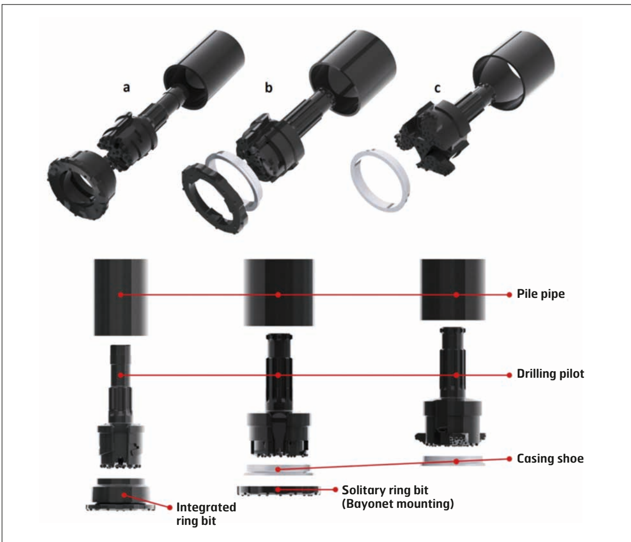
Figure 13. Drilling accessories used in RD pile wall construction (Figure: Robit Oyj)
