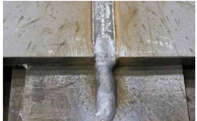
FIGURE 24 Pay attention to the stops, which are placed on the sacrificial plate. This plate is then removed by grinding.
