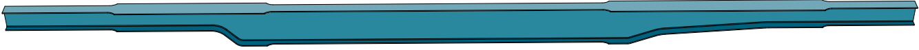
Figure 5 Variable flange width can be introduced to improve the bending resistance and the bending stiffness in critical areas.
