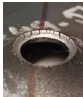
The punched hole in Strenx® 700MC Plus showed no cracks, unlike the S700MC steel.
