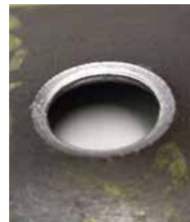
The punched hole in Strenx® 700MC Plus showed no cracks, unlike the S700MC steel.
