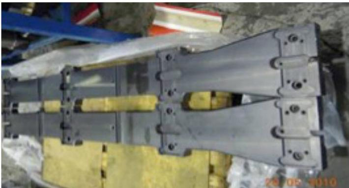
**Fig 1. Toolox® 33 support beams**
