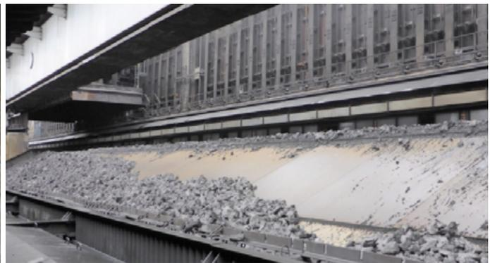
**Fig 4. Cooling bed made in Toolox® 33**
