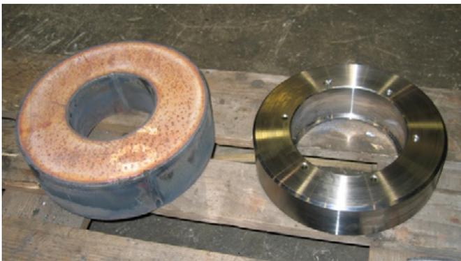
**Fig 3. Toolox® 44 steering wheel**
