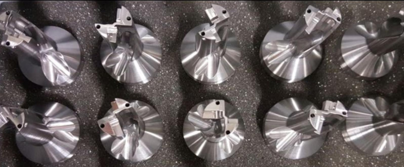
Toolox® is a new steel made by Swedish special steel producer SSAB. Its is delivered with an unique of high mechanical strength and crack resistance. Therefore it is ideal for high performing tooling like U-drills and high speed mills. The high mechanical strength up to 45 HRC takes away the need for heat treatment. Thus shortening lead times and reducing quality problems.
