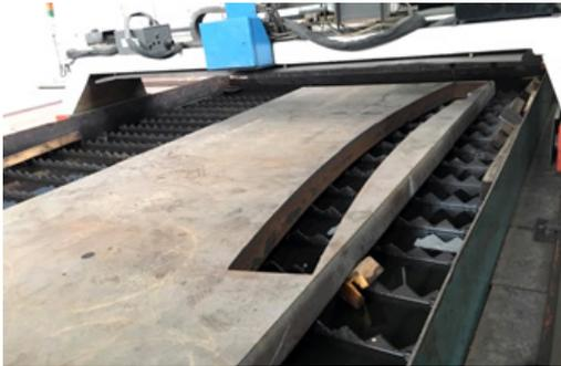
**Fig 1. Oxycutting of Toolox® piece**
