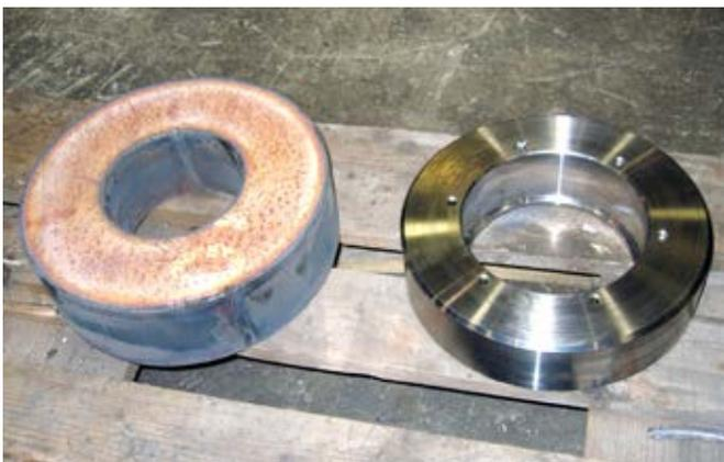
Crane steering wheels in a steel plate rolling mill. The wheels are normally changed every 3-5 years. Previously 35CrNiMo14 (similar to W.Nr.1.6582) machine steel was used. The wheels were induction hardened to a depth of 10 mm. Now Toolox® 44 with no surface treatment is used. Large advantage in manufacturing is achieved since time is saved due to no need of heat treatment. Furthermore, cutting the rings from plate saved machining time and guaranteed a homogeneous small grain structure.
