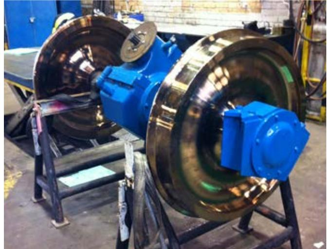
Toolox® maintains a high mechanical resistance up to 600 °C. This is a benefit used in a wagon at a aluminium plant for charging aluminium coils into an annealing oven. The oven holds a temperature at 560 °C, which means that the wheels are repeatedly heated and cooled. Previous material for these wheels was stainless steel, now they have changed to Toolox® 44.
