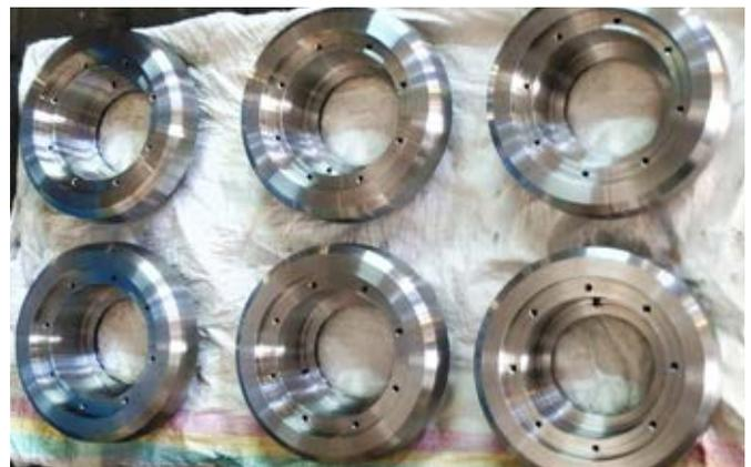
Guide rollers in cement mill stacker/reclaimer. In the previous solution case hardened 42CrMo4 was used. Changing to Toolox® 44 decreased lead time with 10 days due to no need to send the rollers for heat treatment. A much better surface finish with Toolox® gives better resistance to adhesive wear.
