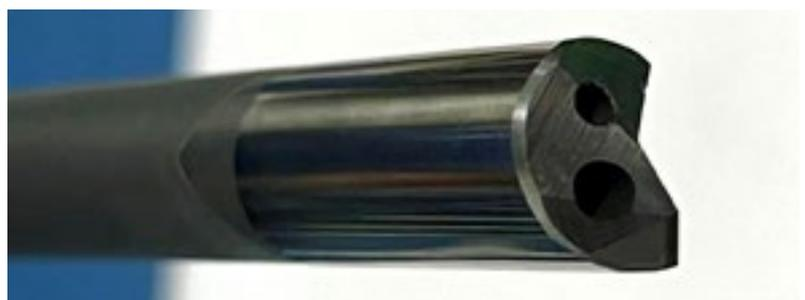
The results from the YuanChang gun drilling testing shows that long holes in Toolox® 44 can be made in a perfect way without any complications. As long as the right parameters are used and top tools are implemented.
