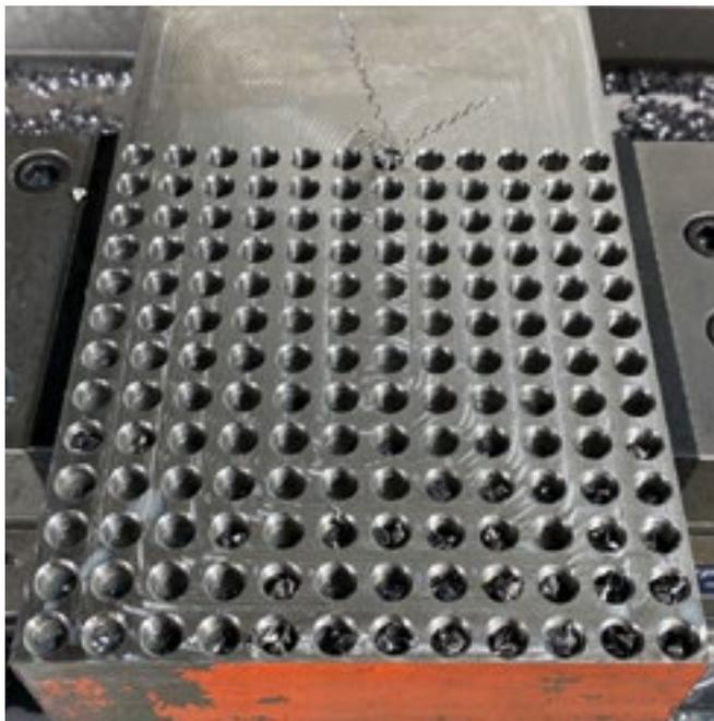
The results from the Sandvik Coromant tapping testing shows that threads in Toolox® 44 can be made in a perfect way without any complications. As long as the right parameters are used and top tools are implemented.
